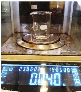
Penimbangan Koagulan Recycle Tawas dosis 80 mg/L
