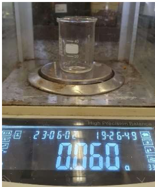
Penimbangan Koagulan Recycle PAC dosis 120 mg/L
