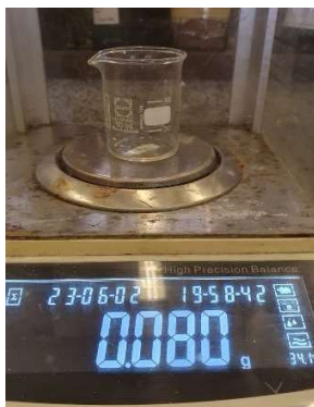
Penimbangan Koagulan Recycle PAC dosis 160 mg/L
