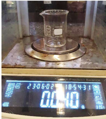
Penimbangan Koagulan Recycle PAC dosis 80 mg/L
