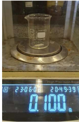
Penimbangan Koagulan Recycle PAC dosis 200 mg/L
