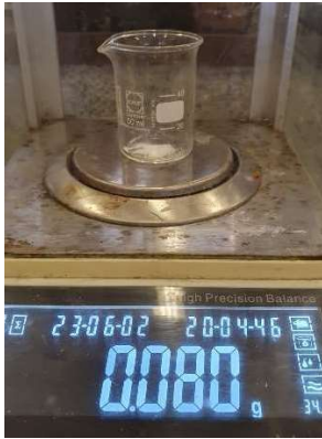
Penimbangan Koagulan Recycle Tawas dosis 160 mg/L
