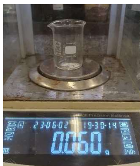
Penimbangan Koagulan Recycle Tawas dosis 120 mg/L
