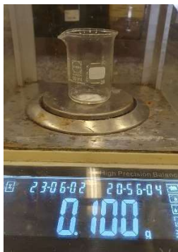
Penimbangan Koagulan Recycle Tawas dosis 200 mg/L
