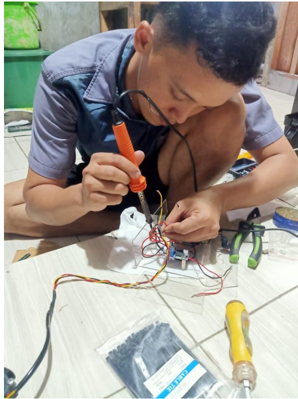
Gambar 2. Proses perakitan alat monitoring air PDAM.
