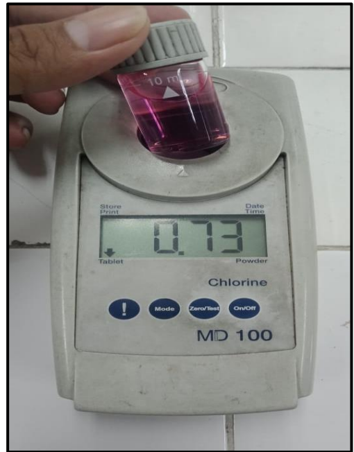
Hasil pengukuran sisa chlor ( \text{Cl}_2 ) 0.73 mg/L
